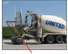
The Pallet Shelf conveniently holds fiber mesh or other additives, in close proximity to the trucks loading chute.
